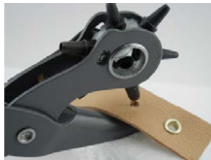
[Photo 2: Punch or cut a hole]
